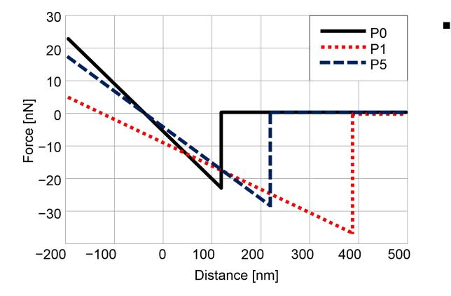
Sample P0 had the highest adhesion force of 24 ± 3 nm and a short activity range, which can be attributed to the relatively smooth and tough oxide surface.
